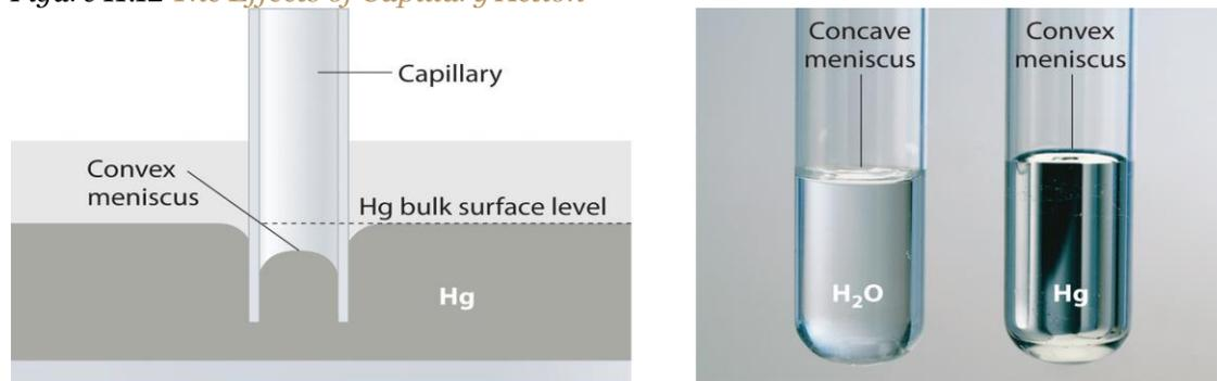
(a) This drawing illustrates the shape of the meniscus and the relative height of a mercury column when a glass capillary is put into liquid mercury. The meniscus is convex and the surface of the liquid inside the tube is lower than the level of the liquid outside the tube. (b) Because water adheres strongly to the polar surface of glass, it has a concave meniscus, whereas mercury, which does not adhere to the glass, has a convex meniscus.
