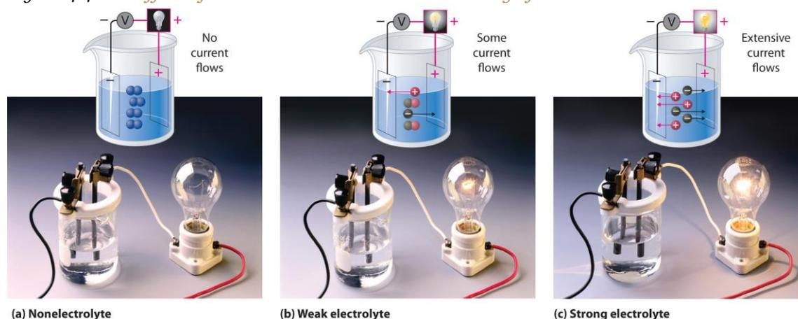
An electrical current will flow and light the bulb only if the solution contains ions. (a) Pure water or an aqueous solution of a nonelectrolyte allows almost no current to flow, and the bulb does not light. (b) A weak electrolyte produces a few ions, allowing some current to flow and the bulb to glow dimly. (c) A strong electrolyte produces many ions, allowing more current to flow and the bulb to shine brightly.
