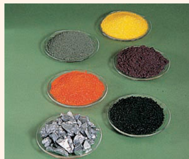
FIGURE 3.9 ▲ Chromium compounds of different colors Clockwise from top: Potassium chromate, \text{K}_2\text{CrO}_4 ; chromium(VI) oxide, \text{CrO}_3 ; chromium(III) sulfate, \text{Cr}_2(\text{SO}_4)_3 ; chromium metal; potassium dichromate, \text{K}_2\text{Cr}_2\text{O}_7 ; chromium(III) oxide, \text{Cr}_2\text{O}_3 .
