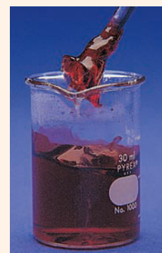
FIGURE 3.5 ▲ Preparing resorcinol-formaldehyde plastic
