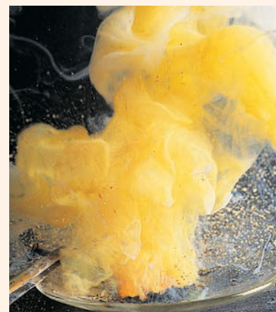
FIGURE 3.16 ▲ Reaction of zinc and sulfur
