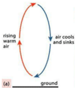
In a convection cell, warm material rises and cool material sinks. In mantle convection, the heat source is the core.
